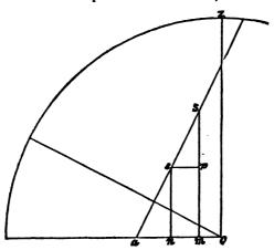
diurnal circle on which S and s are the Sun's two places at different times and S m and s n the S'ANKUS or the sines of altitudes of the Sun, then O m, n n will be the BHUJAS, n m or s p the difference between the BHUJAS and S p the difference between the s'ANKUS.
