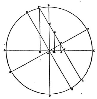
Let BODE be meridian of the given place, CAE the diameter of the Horizon, B the Zenith, P and Q the north and south poles, B A D the diameter of the Prime Vertical, F A G that of the Equinoctial, P A Q that of the six o'clock line, H f L that of one of the diurnal circles, s the Sun's projected place in it and f h, s m, H n perpendiculars to O E. Then
