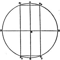
3. The versed sine is like the arrow intersecting the bow and the string, or the arc and the sine.\*
