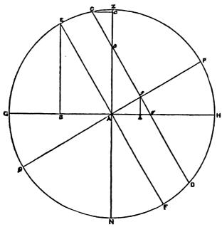
Let Z G N H be the meridian of the given place, G A H the diameter of the horizon, Z the Zenith, P and Q the north and south poles, E A F the diameter of the equinoctial, P A Q that of the six o'clock line, O f D that of one of the diarnal circles, and E B, f h the perpendiculars to G II. Then it is clear from this that
