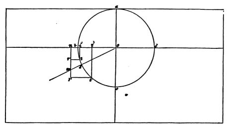
• In the accompanying diagram of the PHALAKA YANTEA, o is the centre of the circle a b o and the line o s passing through o is called MADHYAJKA' or middle sine. If the shadow of the pin touches the circumference in S when the instrument is held in the vertical circle passing through the Sun, S b will then be the zenith distance of the Sun. From this the time to or after midday can be found in the following manner.
