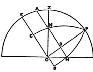
\* First of all assume H N the TAD-DURITI = sine of the given elevated time that is = sin 80°. From this find the S'ANKU or the sine of altitude by similar triangles.
