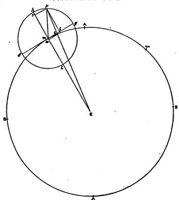
[In fig. 2, let A B C D be the concentric, T the place of the stellar Aries, E the centre of the Earth, M the mean place of the planet in the doncentric, h f l g, the Epicycle, h the place of the higher apsis in it, E h the UCHCHA-RERHA' l the place of the lower apsis, P that of the planet, h P the KEEDHA, P k the sine of the KENDHA and P i the cosine of it.
