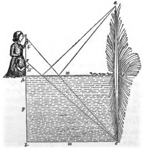
• Let df = fc = height of bamboo = kb then b a or y = height of bamboo and man's height together. Let b c = breadth of water = x then by first observation
